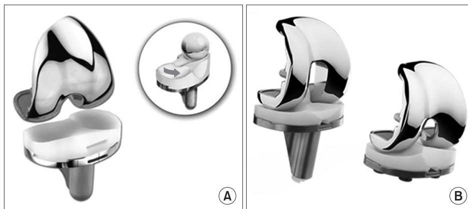
Fig. 1. (A) Photograph of the medial pivot knee showing a deeper and more medial surface of the articular insert that articulates with a congruent medial femoral condyle and the anterior lip that provides stability in flexion and a less congruent lateral surface that allows free movement of lateral femoral condyle along an arcuate path. (B) Photograph showing the posterior-stabilized design with a cam and post mechanism with symmetrical, minimally conforming, articular insert and a post to engage the cam in the femoral condyle and ensure rollback.
